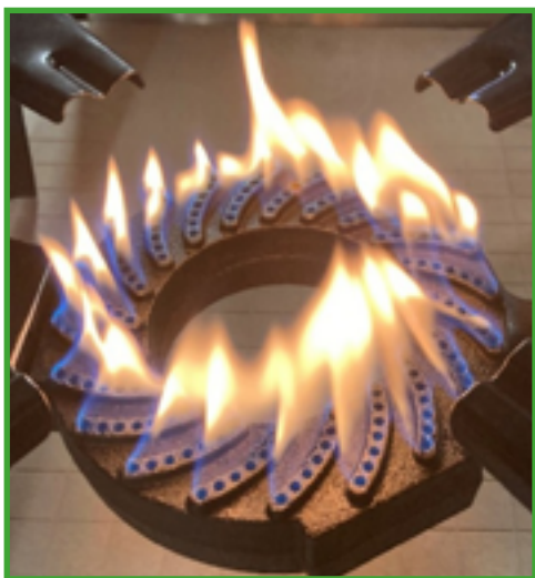
A yellow wispy flame due to insufficient air.
